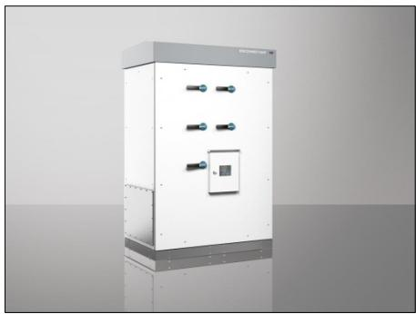
The Disconnect Unit provides maximum safety by disconnecting the direct current (DC) input and alternating current (AC) output from the inverter in case of maintenance or emergency. Load-break switches are mounted on a single switchboard, working under full load conditions and ampacity reserves required by NEC 2011. Lockable switch handles are located on the front of the cabinet, making it easy to identify switch status.
