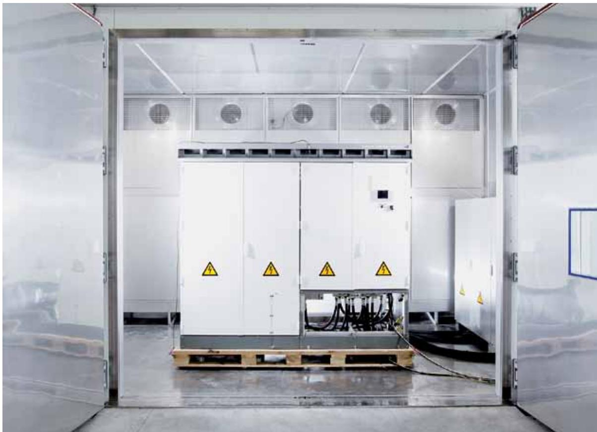
The chamber can also create relative humidity of between 10 percent and 95 percent. The inverters are subjected to these kinds of conditions in tests lasting up to 1,000 hours under constant conditions.
